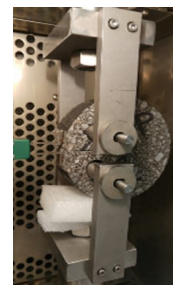
Testing apparatus to evaluate asphalt cracking
