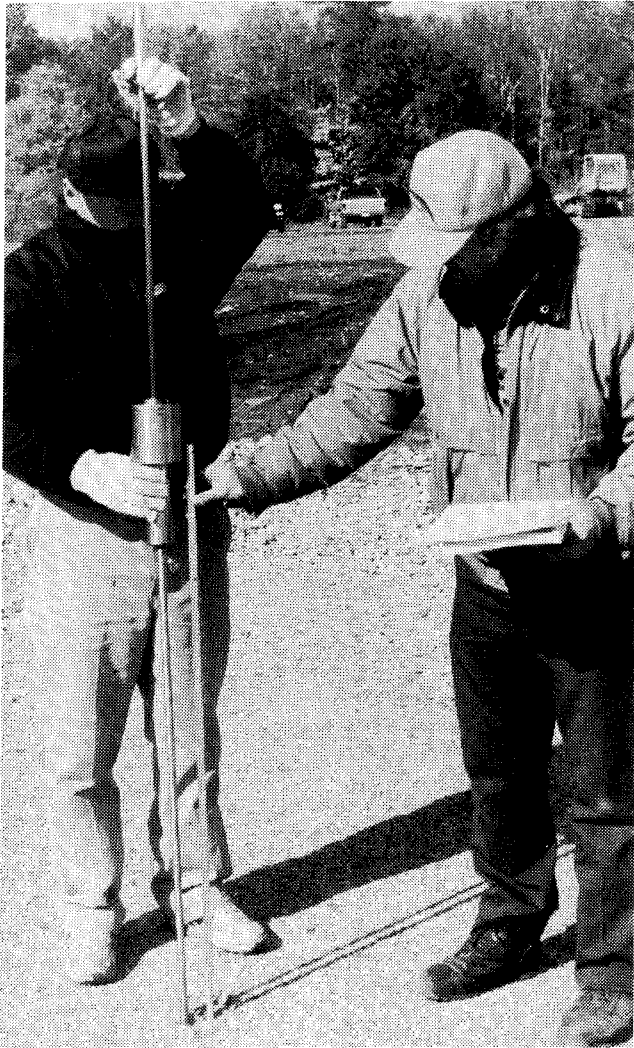
Figure 7. Dynamic Cone Penetrometer (DCP).
