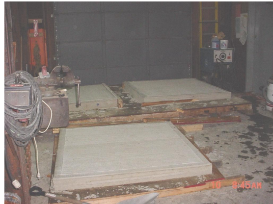
Concrete panel fabrication in the Bridge Maintenance Bureau shop
