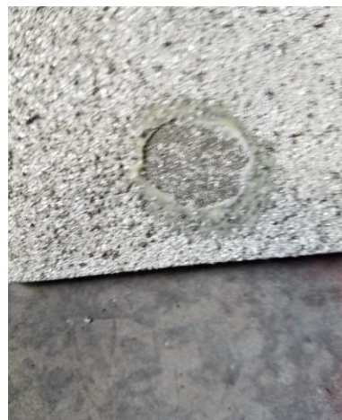
Adhesion Test Result (08/12/2016 Companion Plate, Dollie No. 3)
