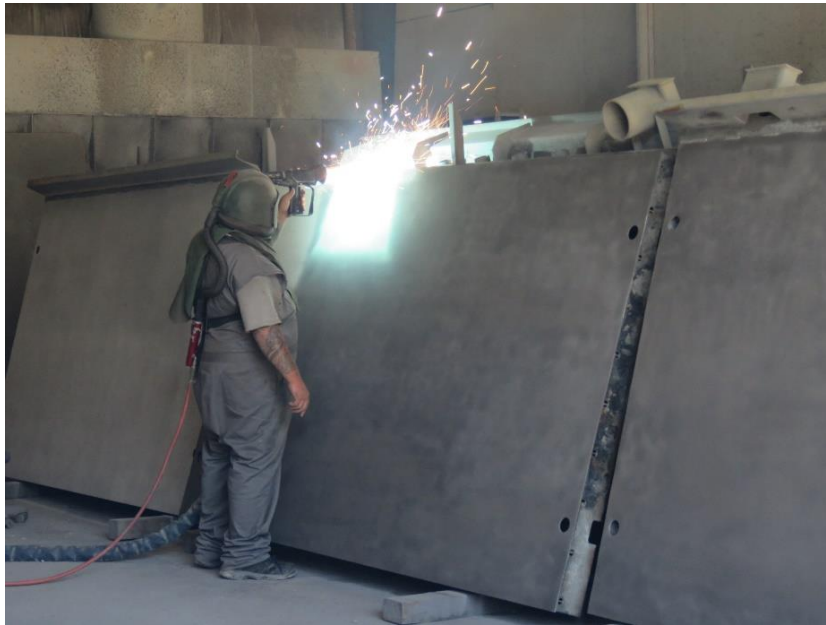
Figure 2. SafTrax coating process performed by Excelerated Coatings in Epsom, NH
