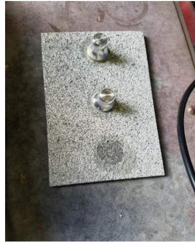
Adhesion Test Result (08/12/2016 Companion Plate, Dollie No. 1)
