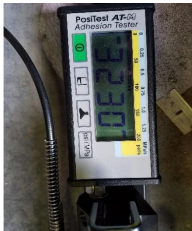
Adhesion Test Result (08/12/2016 Companion Plate, Dollie No. 2)
