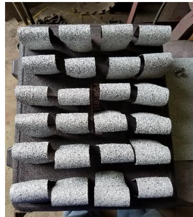
Bend Tabs Inspected
