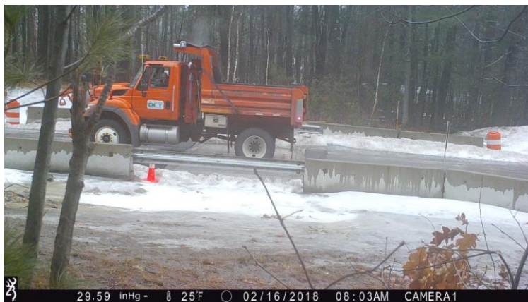
Figure 3: Sample image from trail camera used to obtain estimate of traffic volume.
