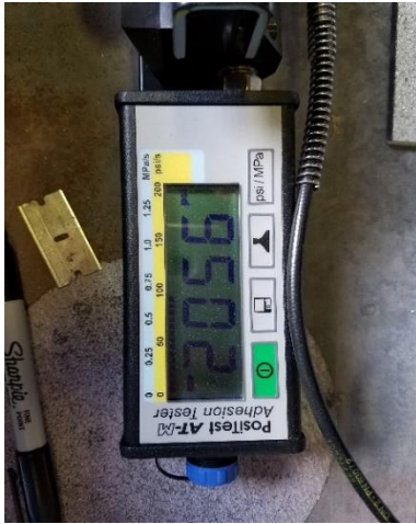
Adhesion Test Result (08/12/2016 Companion Plate, Dollie No. 1)
