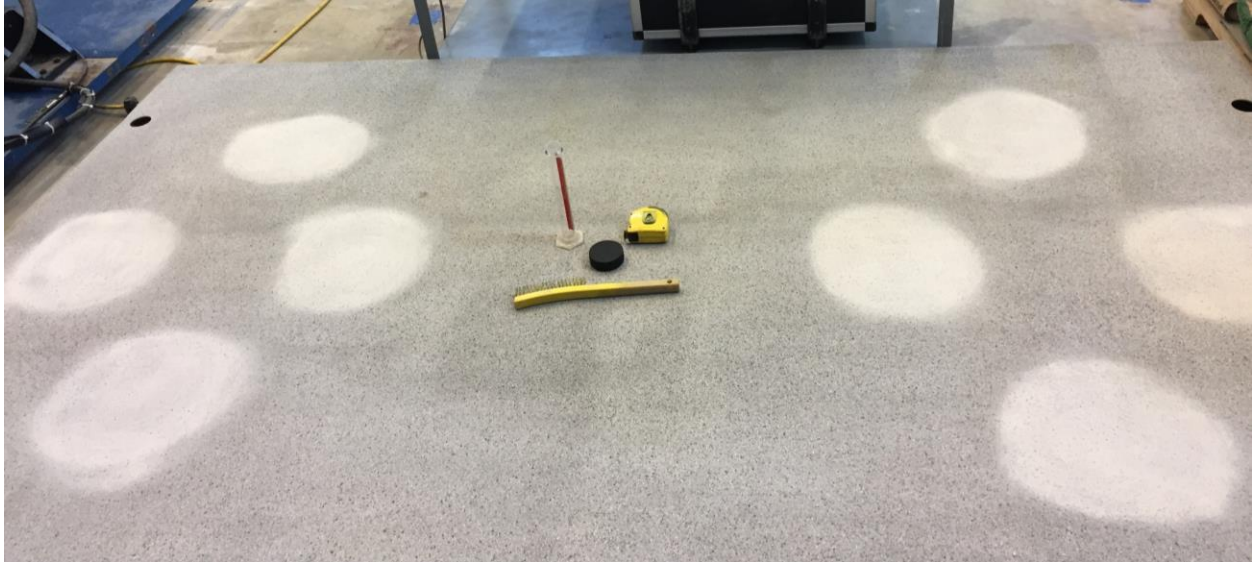
Figure 3: Post macrotexture depth testing.
