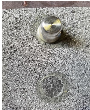
Adhesion Test Result (08/12/2016 Companion Plate, Dollie No. 2)
