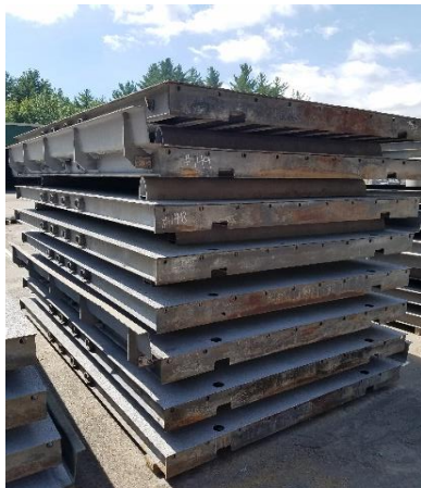
Stacked Deck Panels (Completed)
