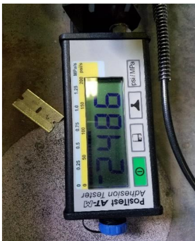
Adhesion Test Result (08/12/2016 Companion Plate, Dollie No. 3)
