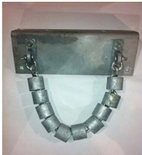
Figure 54. Chain mooring system.
