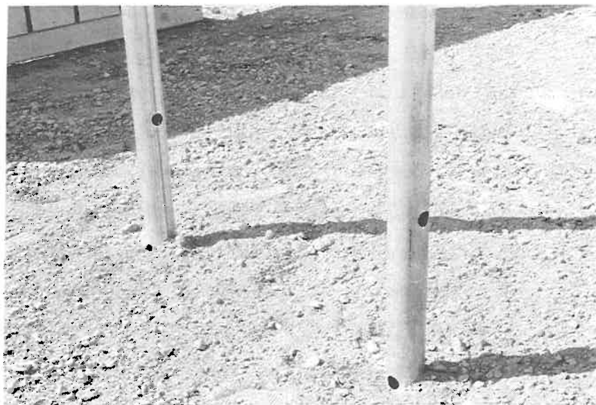
Figure 99 . Dual 4 in. aluminum sign support installation modified with four - 1.5 in. holes and anchored in strong soil (test 405231-16).
