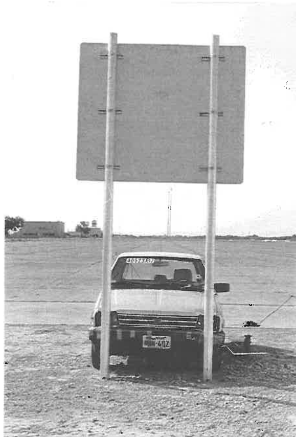
Figure 104 . Vehicle/sign installation geometrics for test 405231-17.
