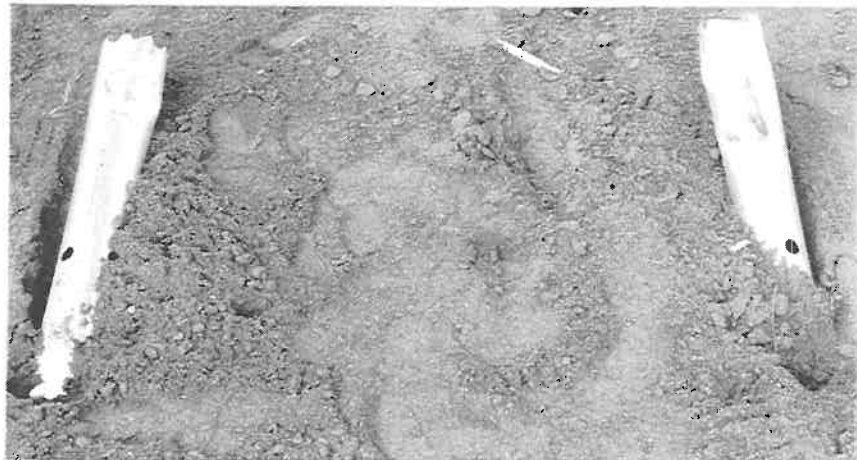
Figure 171. Dual 4-in with 1-in holes aluminum sign support anchored in weak soil after test 405231-26.
