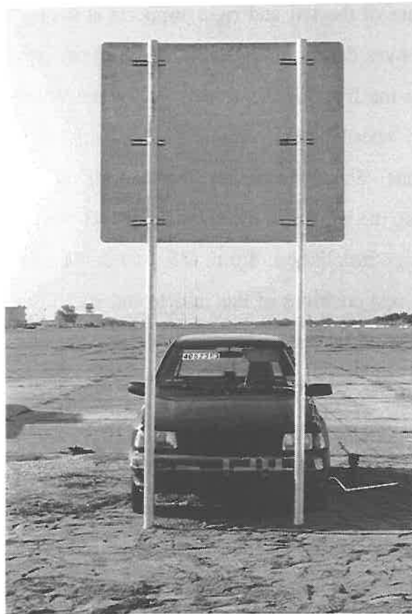
Figure 22 . Vehicle/sign installation geometrics for test 405231-3.
