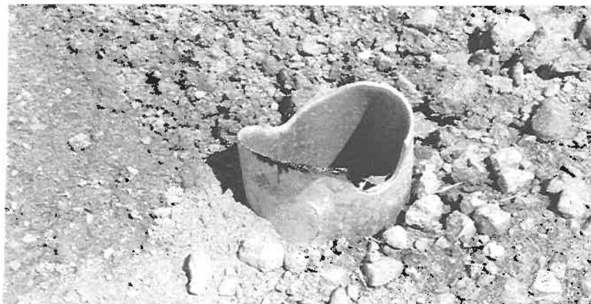
Figure 108. Dual 4 in. aluminum sign support installation modified with four - 1.5 in. holes and anchored in strong soil after test 405231-17.
