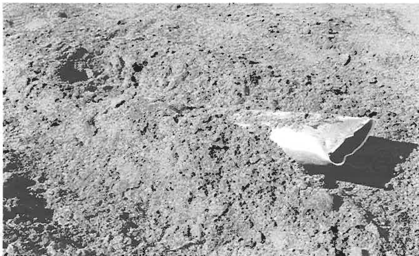
Figure 57 . Single 4 in. aluminum sign support installation anchored in weak soil after test 405231-8.
