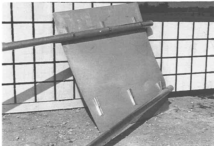
Figure 38 . Dual 4 in. aluminum sign support installation anchored in strong soil after test 405231-5.
