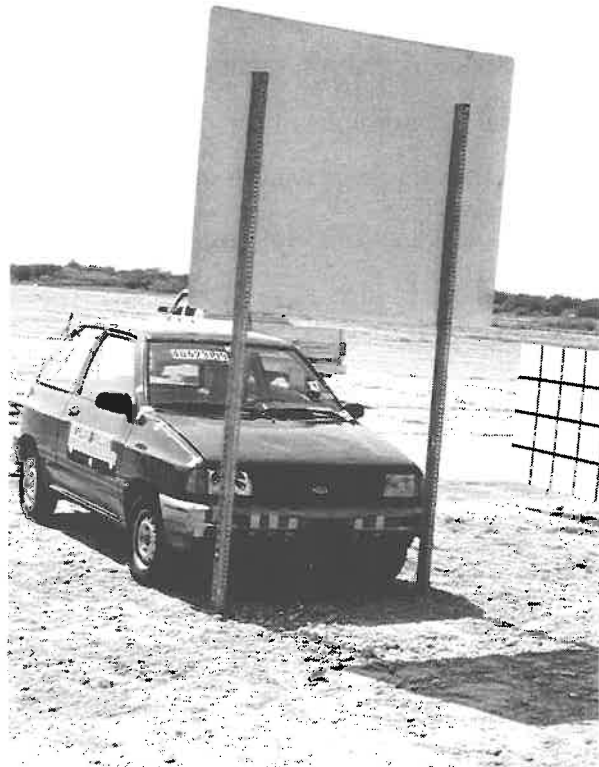
Figure 118. Vehicle/sign installation geometrics for test 405231-19.
