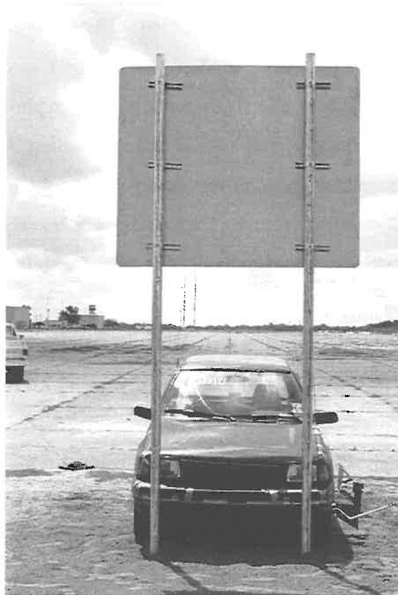
Figure 29 . Vehicle/sign installation geometrics for test 405231-4.
