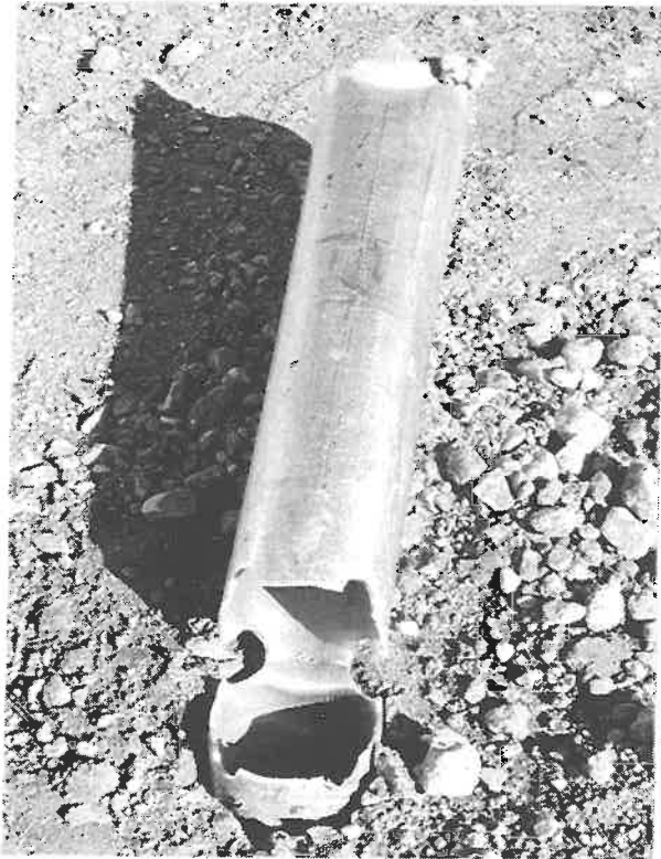
Figure 150 . Dual 4-in with 1-in holes aluminum sign support installation anchored in strong soil after test 405231-23.
