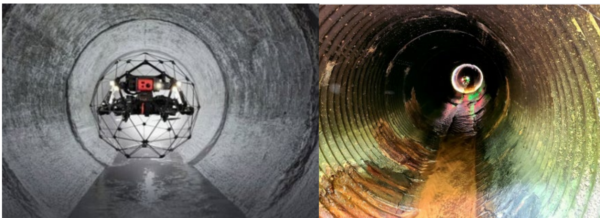
Figure 14. Flyability Elios 2 UAS Conducting Maryland DOT Culvert Inspection.
