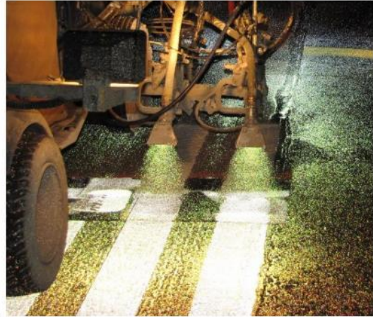
Picture 2 – glass bead guns adjusted.
