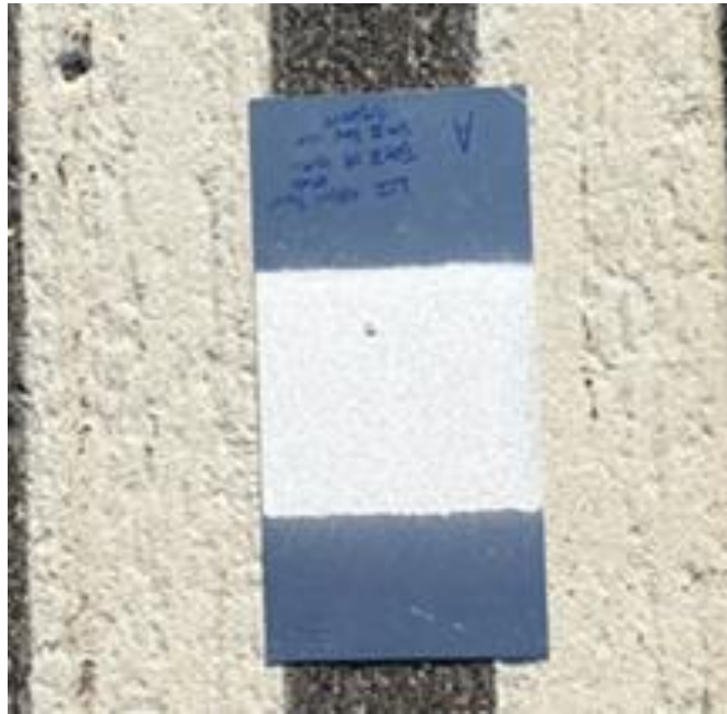
Figure 16: Control Sample Placed Next to Field Paint
