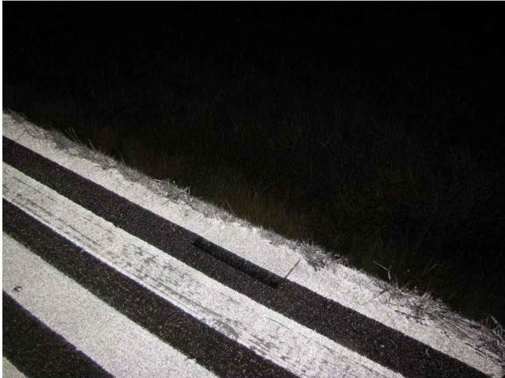
Picture 5 – Test panel placed longitudinally along outer line closest to the grass.
