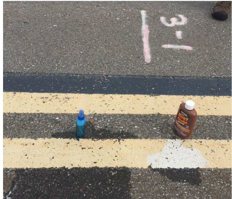
Figure 21: Soap and Water vs. Rust Remover
