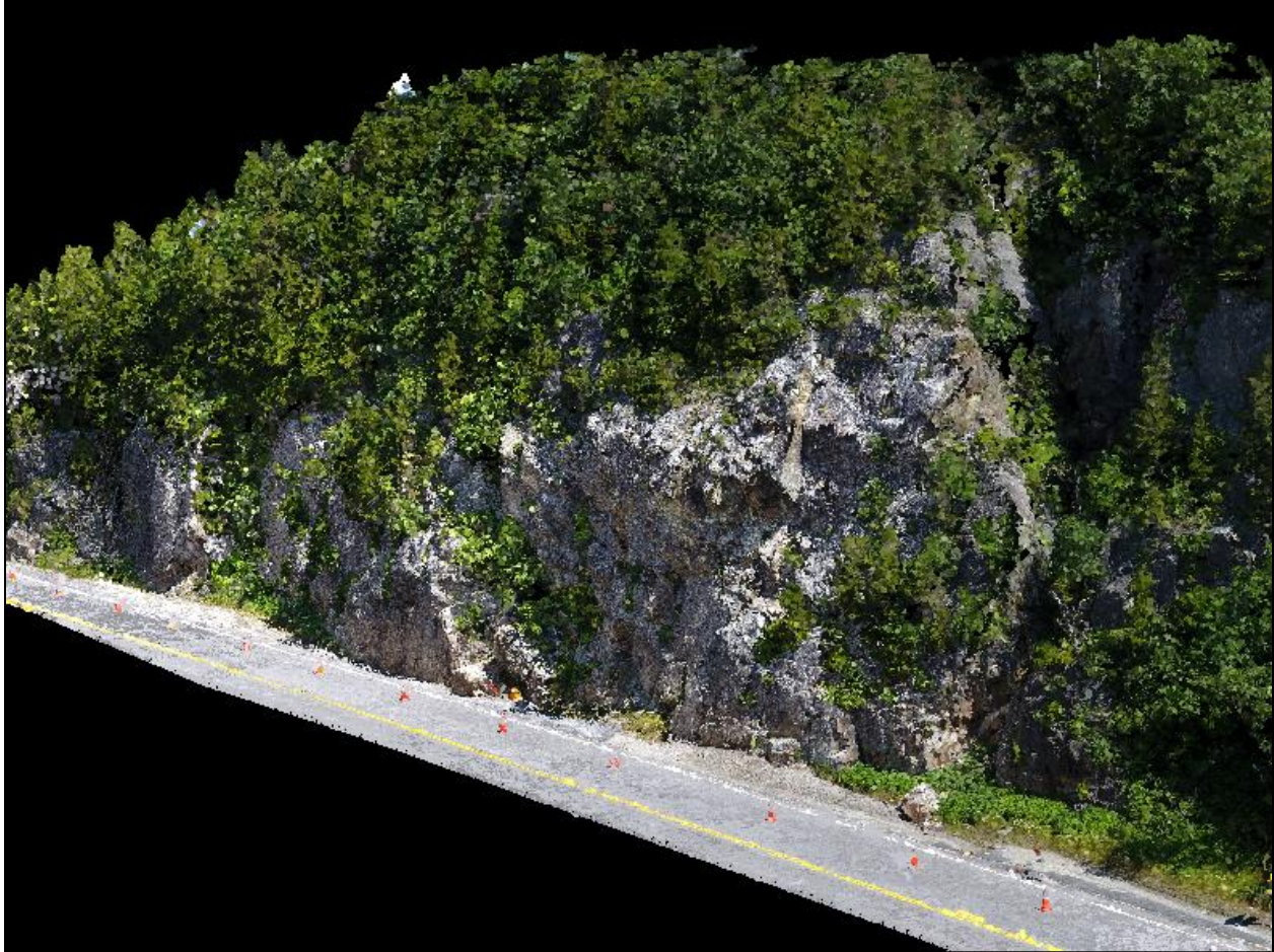
Figure 40. The 3D point cloud produced during this case study. This data was also uploaded to Sketchfab.
