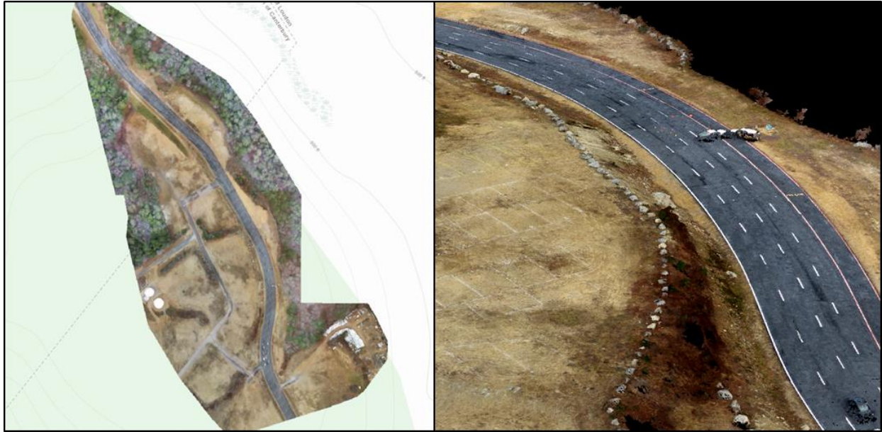
Figure 15. Geospatial products of the accident case study. The orthomosaic imagery is on the left and the 3D point cloud is on the right.
