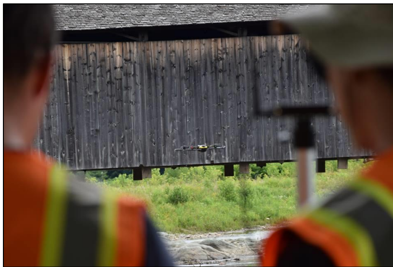
Figure 8. The senseFly Albris in manual operation mode while carrying out a close-range inspection of a historic covered bridge.
