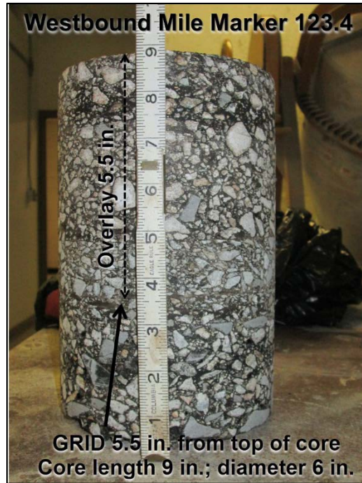
Figure 20. Asphalt core for WB MM 123.4.
