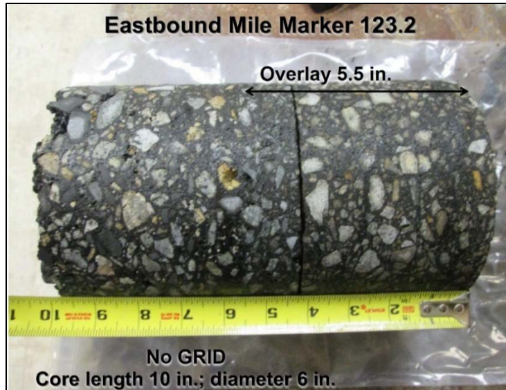
Figure 18. Asphalt core for EB MM 123.2 (no grid reinforcement).
