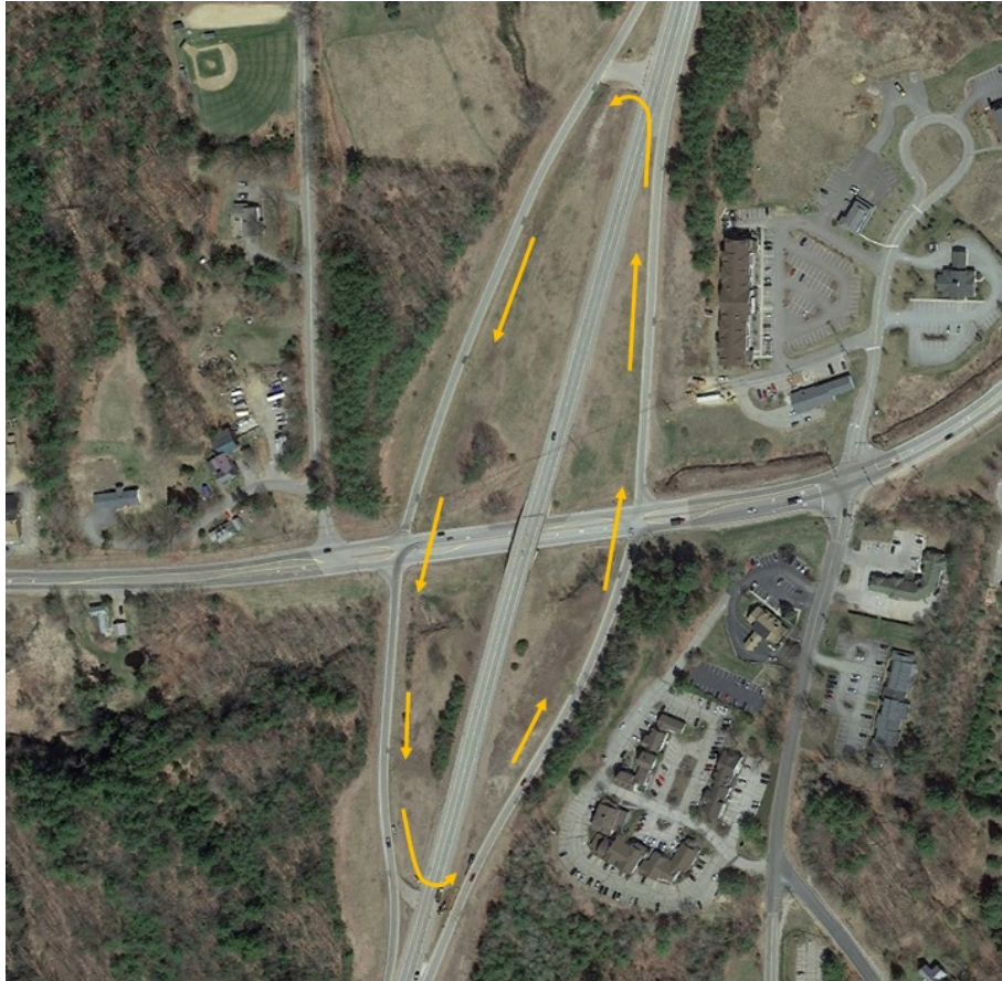
Figure 7 - Proposed traffic flow around the work zone (center).
