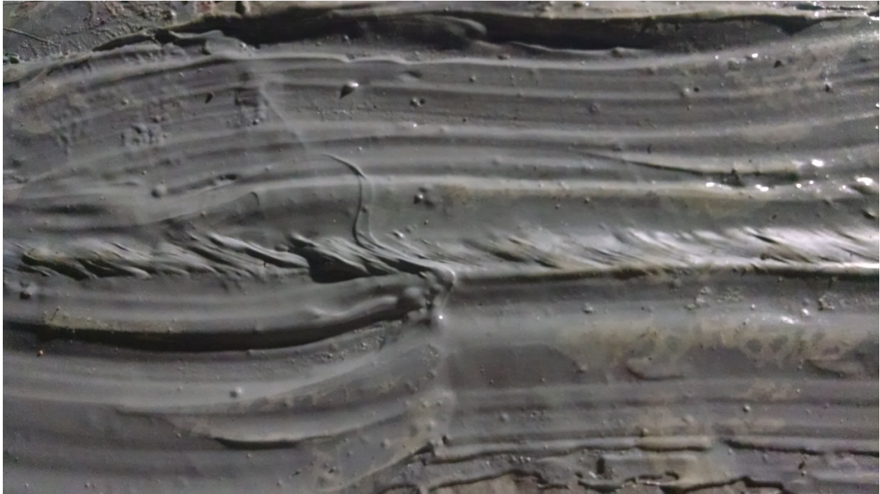
Figure 22 - Joint 1 polymer striation.
