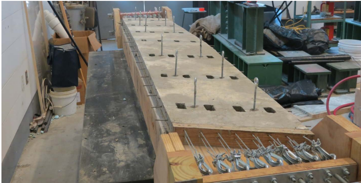
Figure 6 – Panel scale model showing prestressing cables.
