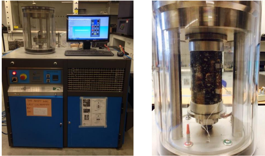
Figure 3- Asphalt Mixture Performance Tester (AMPT) and Complex Modulus Testing Configuration
