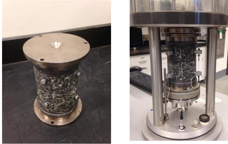
Figure 4- Uniaxial Fatigue Testing Specimen and the configuration in AMPT
