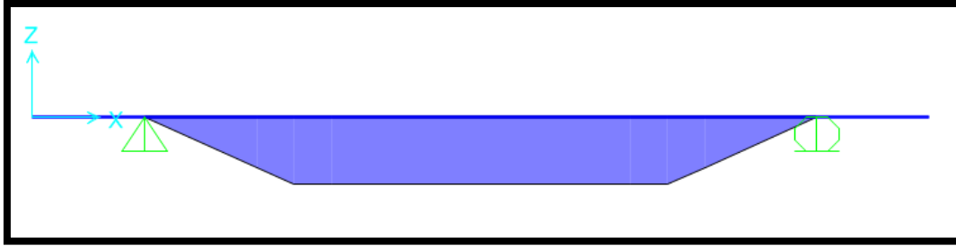
Figure 75: Moment diagram of the laboratory test apparatus (SAP2000, 2014)
