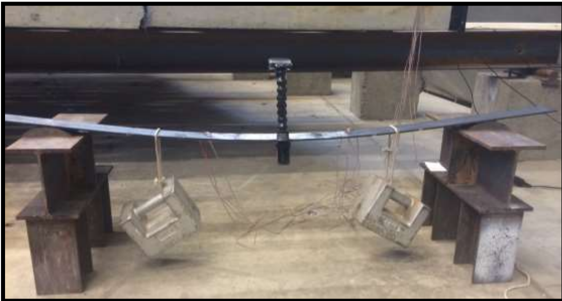
Figure 72: Experimental test apparatus as seen while loaded
