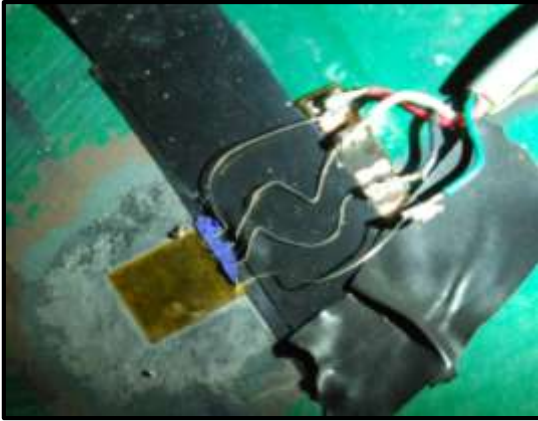
Figure C-13: Photo of Gauge Installation – Soldered Using Terminal Strip
