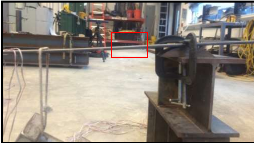
Figure 77: Photo showing the point of inflection in the curvature of the test beam under fixed conditions
