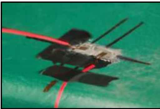
Figure C-20: Photo of Gauge Installation – Quarter Bridge Gauges
