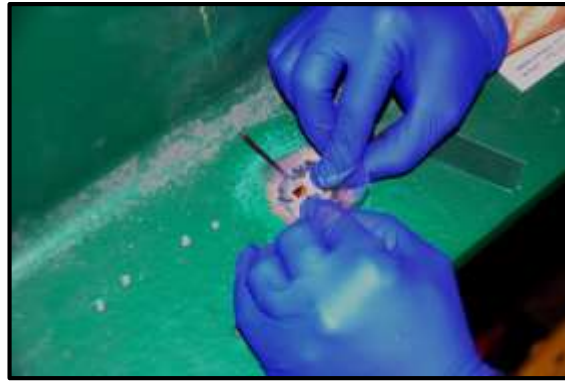
Figure C-11: Photo of Gauge Installation – Tape Removal
