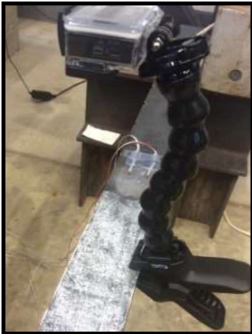
Figure 69: Assembled GoPro® DIC sensor for 2D strain collection
