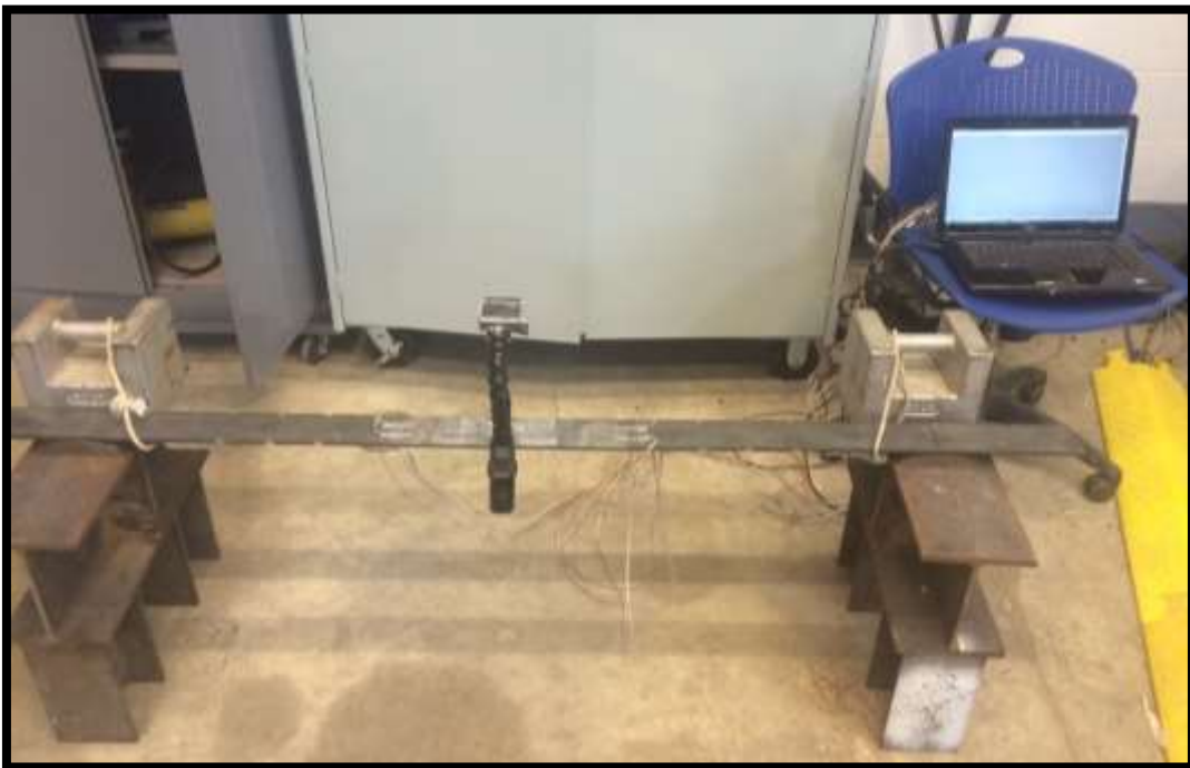
Figure 79: Fully assembled lab testing apparatus showing both the GoPro® DIC and foil gauge strain measurement systems
