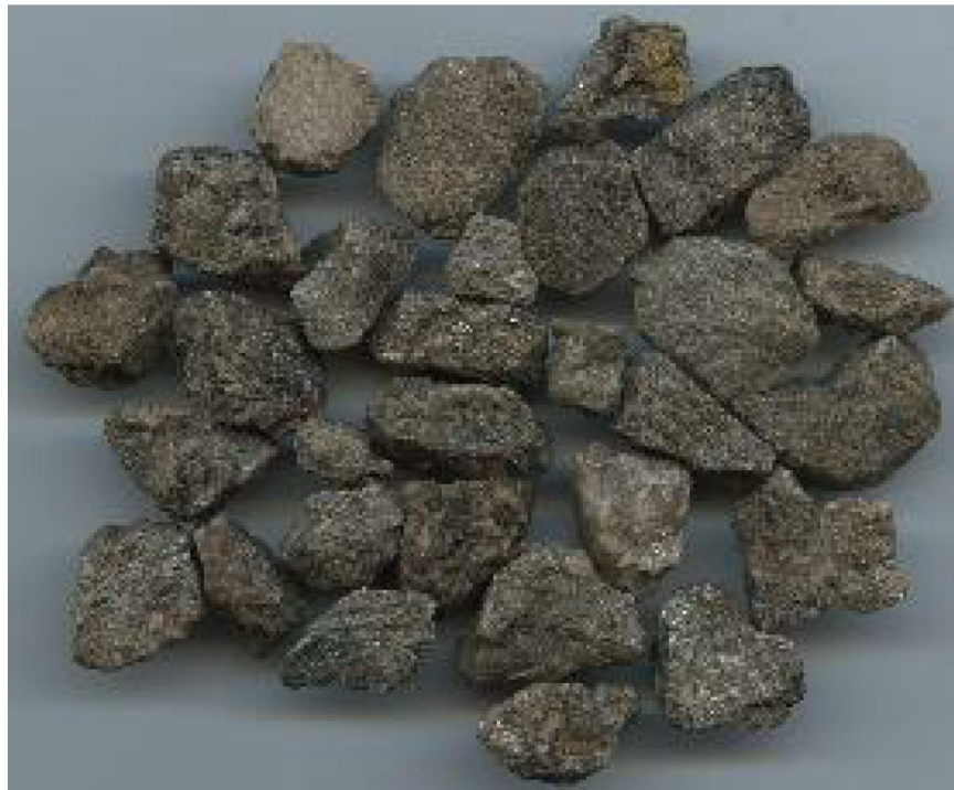
Figure 84 Laconia magnetic aggregates
