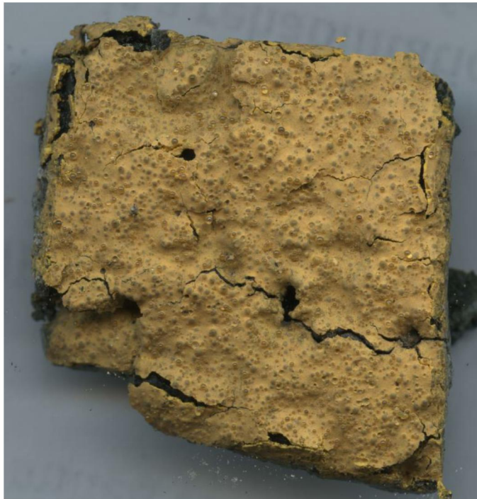
Figure 4 Claremont paint chip showing uniform iron stain coating
