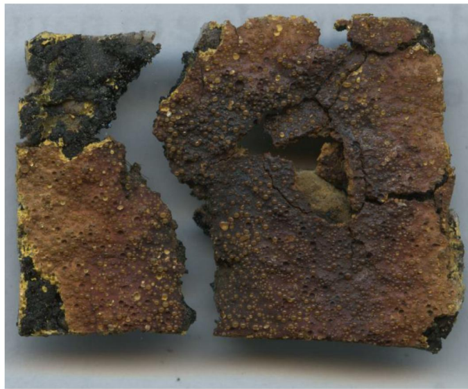
Figure 23 Whitefield paint chip showing large area where staining emerged
