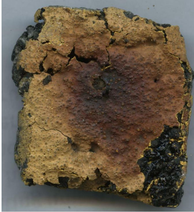
Figure 3 Claremont paint chip showing source of iron stain
