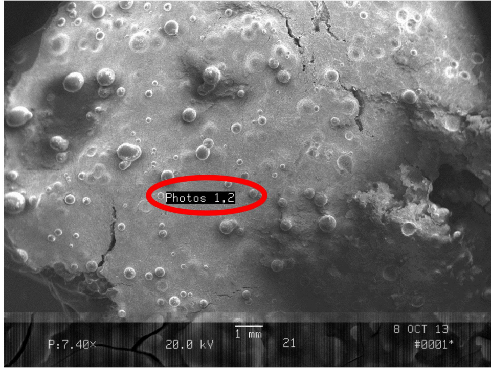
Figure 46 SEM photo of Claremont paint chip showing investigated areas 1 and 2
