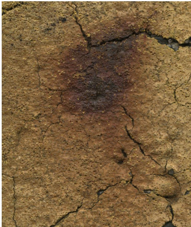
Figure 27 Whitefield close up of Figure 26 note intensity of light color of paint under glass beads lost during coring
