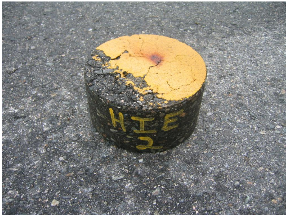
Photo 15 - HIE Core 2 from hold short marking taxiway A at runway 10 right side
