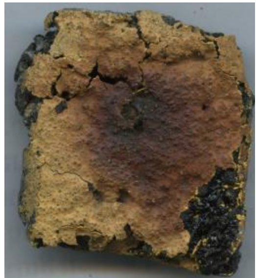
Figure 9 - Sample Rust Stained Paint Chip
