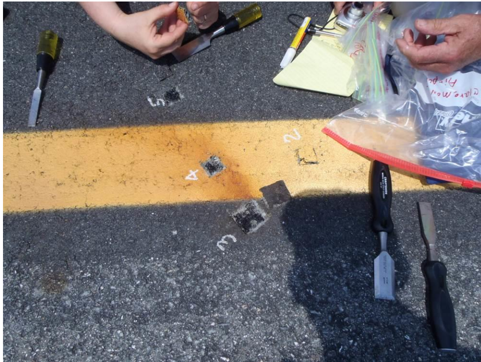
Photo 5 – Paint sample 2 located on no stained paint. Paint sample locations 3, 4 and 5. Sample 3 up gradient, 4 on the paint and 5 down gradient.
