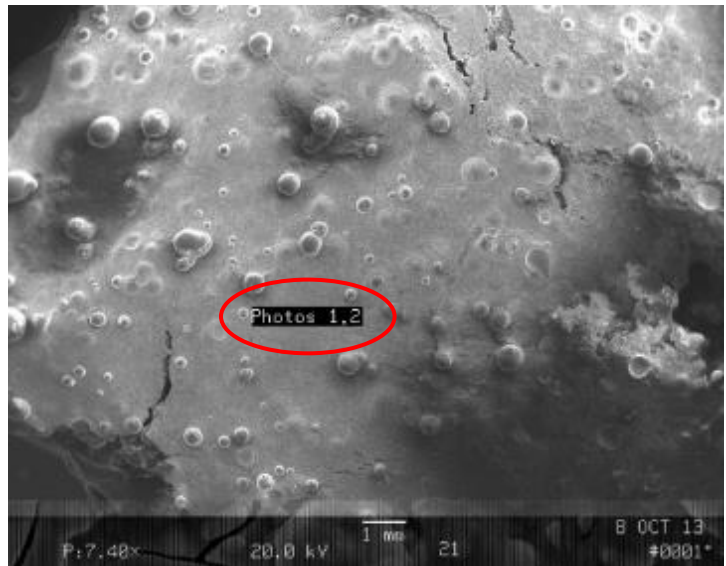
Figure 5 – Sample SEM Photograph of Paint Chip
