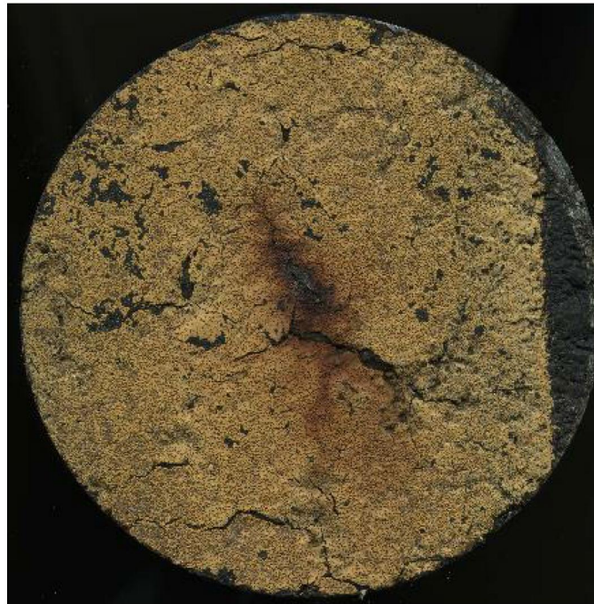
Figure 12 Keene core showing source of iron staining
