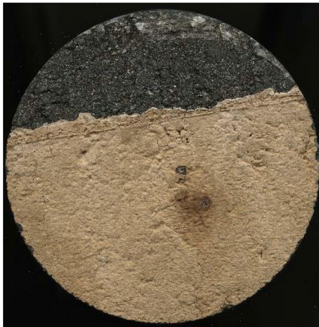
Figure 14 Keene core showing source of stain area
