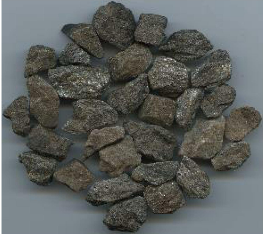
Figure 83 Keene magnetic aggregates
