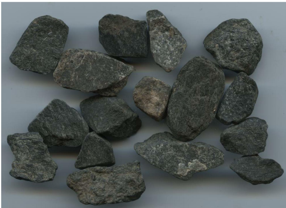
Figure 82 Claremont magnetic aggregates
