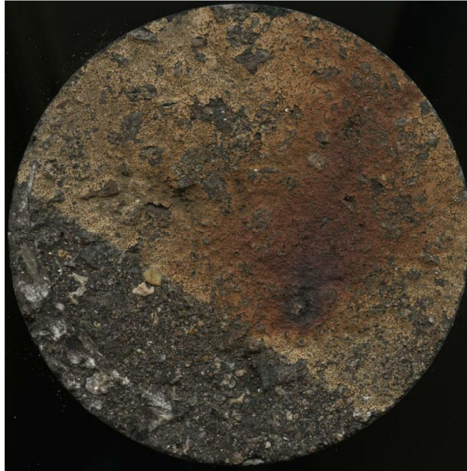
Figure 20 Laconia core showing source of iron staining
