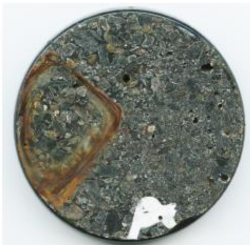
Figure 8- Laboratory Aging Test Rust Stain
