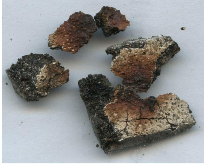
Figure 18 Laconia paint chips showing source of iron staining
