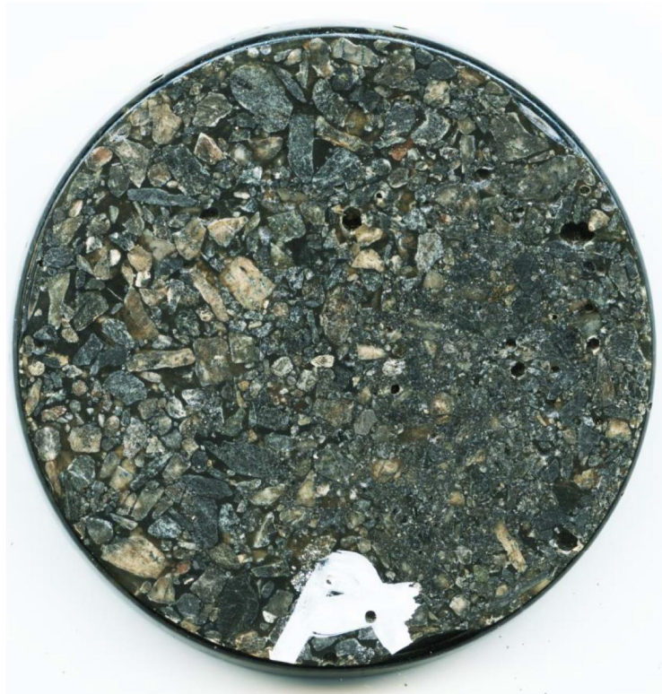
Figure 86 Claremont magnetic aggregate epoxy disk side A after polished in ethanol alcohol
