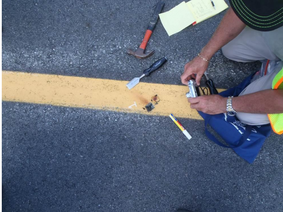
Photo 3 – Paint sample 1 after being removed.
