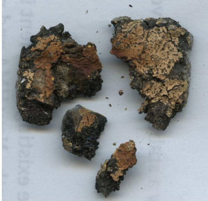
Figure 16 Laconia paint chips showing iron staining
