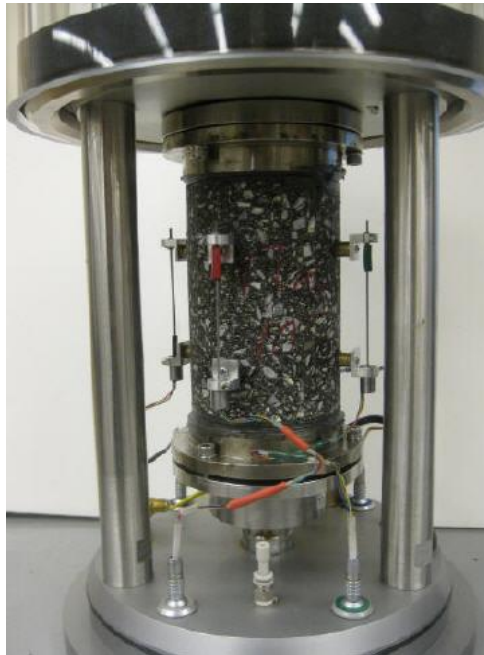
Figure 2.6 LVDT mounting and spacing for SVECD Fatigue
