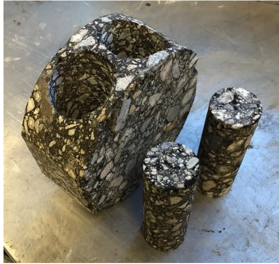
Figure 2.4 Two small specimens produced from one field core
