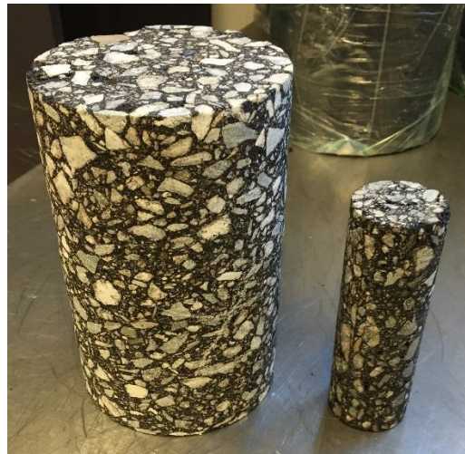
Figure 2.5 Comparison of standard size (left) vs. small geometry specimens (right)
