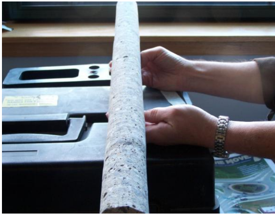
Figure 15: N3P7 CC 17-18 ft depth (several voids)
