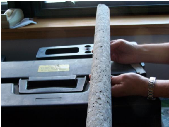
Figure 12: N3P3 SCC 17-18 ft depth (several voids)
