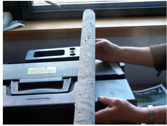
Figure 16: N3P7 CC 26-27 ft depth (more voids)
