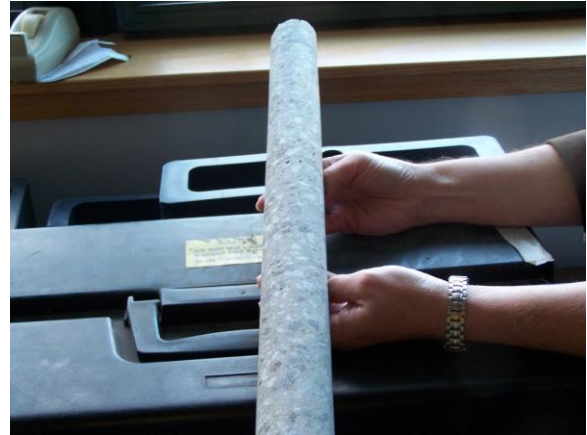
Figure 13: N3P3 SCC 26-27 (less voids)
