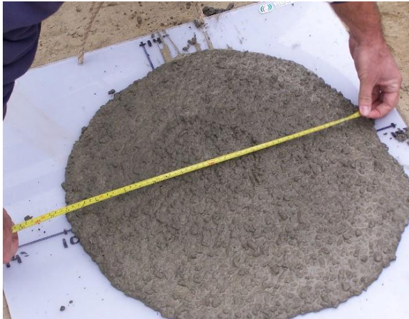
Figure 5: Measuring the spread of SCC
