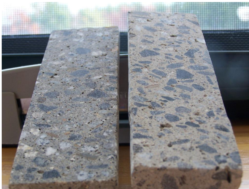
Figure 19: Sections from the 23-foot depth of the piles (SCC on left, CC on right). This was the section with the lowest air content for both piles.
