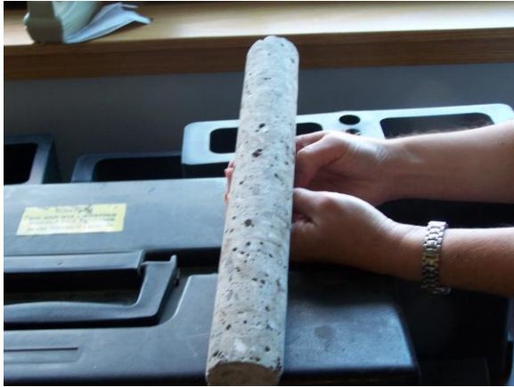
Figure 11: N3P3 SCC 1 to 3 ft depth (more voids)
