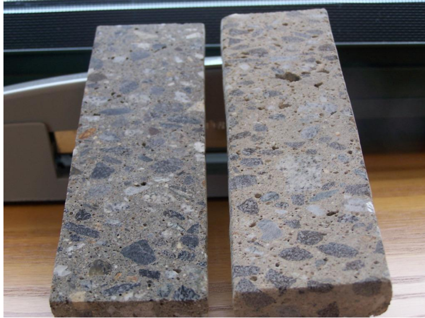
Figure 20: Sections from the 28-foot depth (SCC on left, CC on Right.). This was the section with the highest air content for the CC pile.
