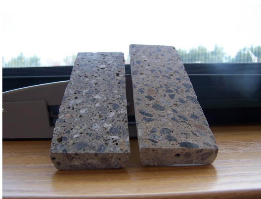
Figure 18: Sections from the 1-foot depth of the piles (SCC on left, CC on right) this was the section of the SCC pile with the highest air content.
