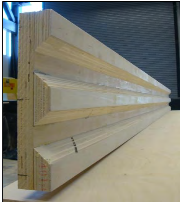
Figure 30: Angular corrugated to form
