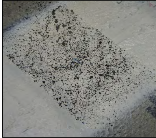
Figure 47: Typical speckle pattern applied for use with DIC system
