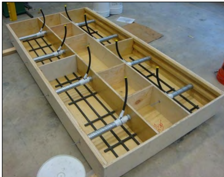
Figure 27: Typical test specimen formwork
