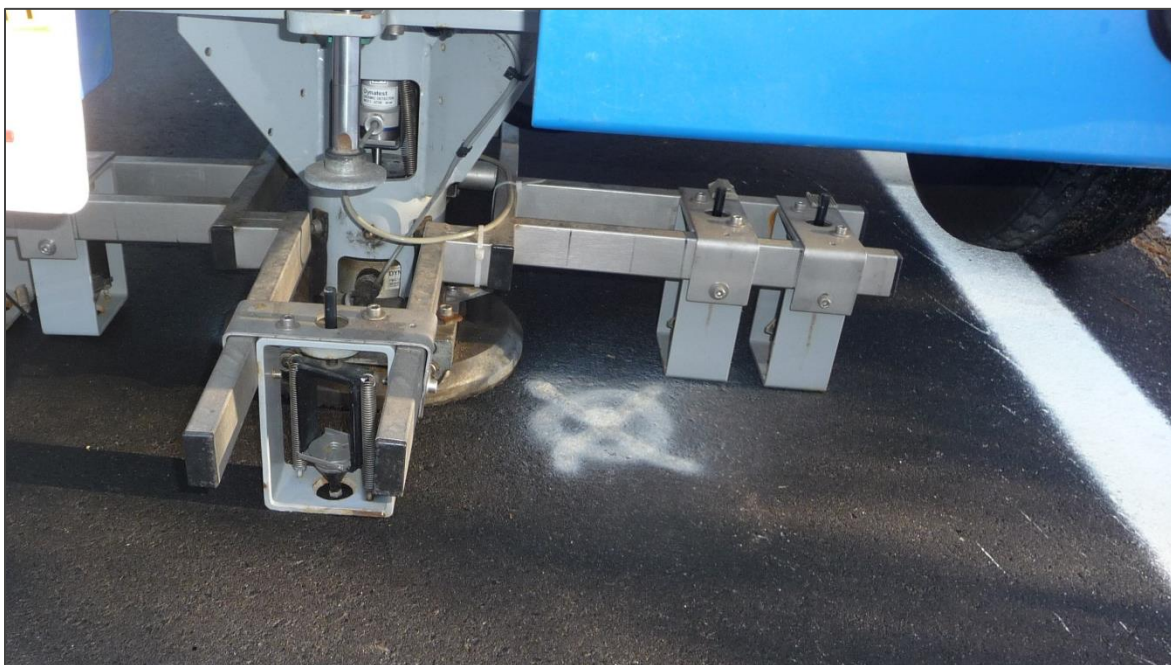
Figure 86: The CP-15 load plate being positioned over a pre-determined wheelpath testing location.
