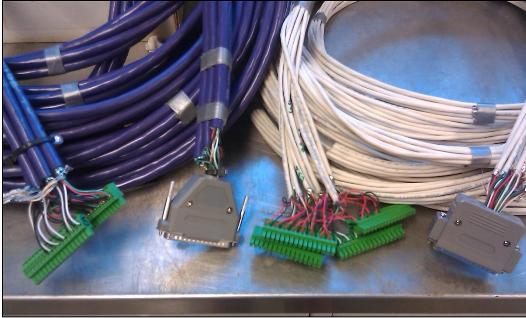
Figure 27: Custom extension cabling for data acquisition.
