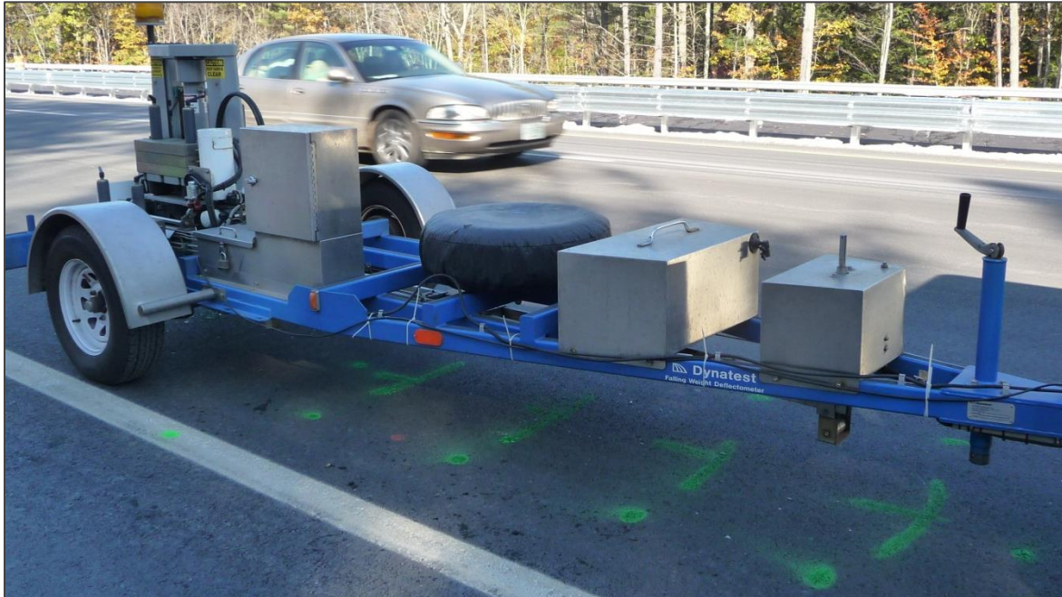
Figure 85: The CP-15 FWD being positioned over the location of subsurface instrumentation.
