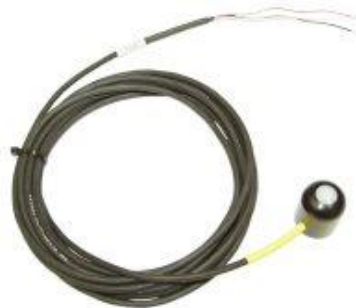
Figure 10: CS 300 pyranometer and lead cables.
