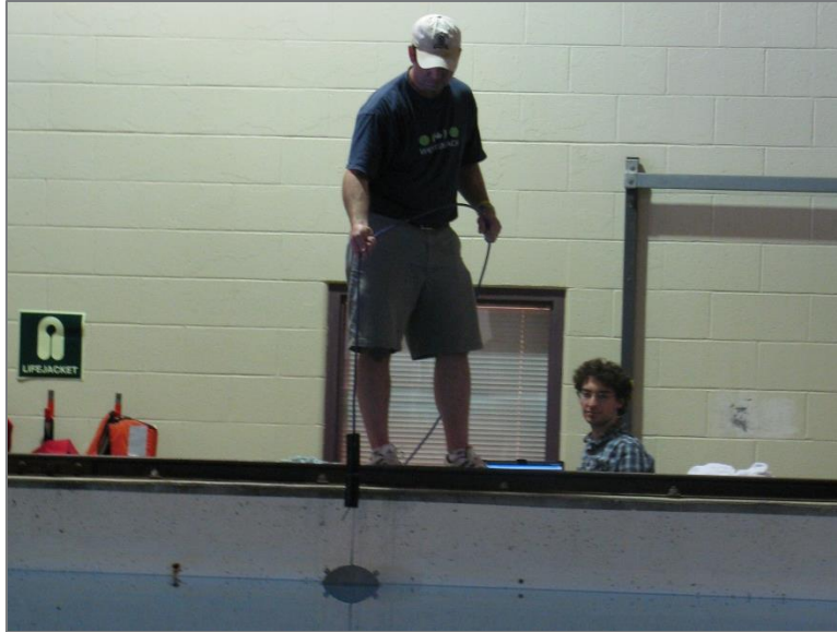
Figure 23: Geokon cell being manually lowered into the engineering pool during initial testing.
