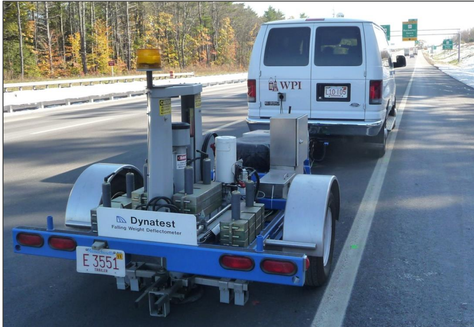
Figure 83: Dynatest CP-15 FWD trailer and the WPI Pavement Research Laboratory van.
