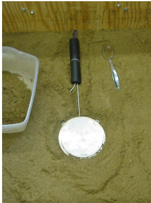
Figure 25: EPC placed in test pit.
