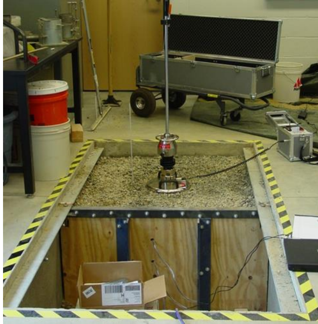
Figure 26: LWD testing being conducted.
