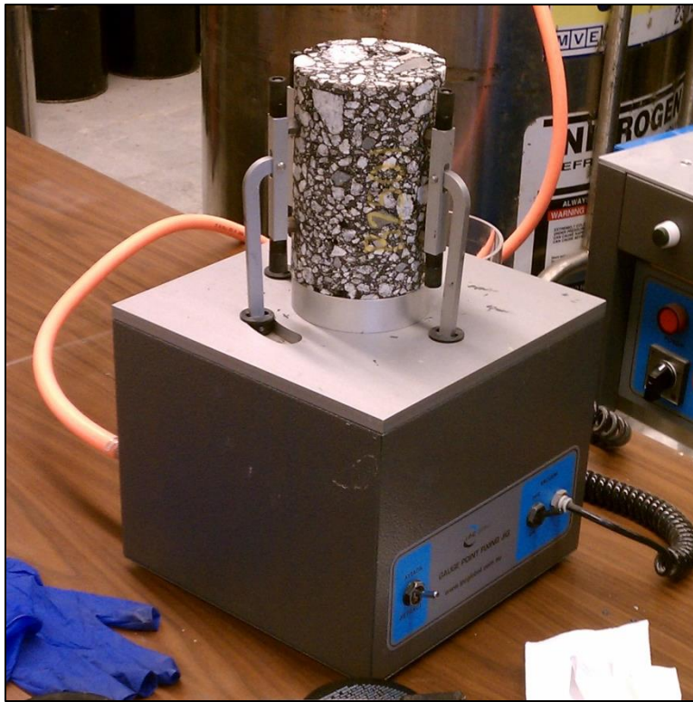
Figure 41: Cut and cored specimen with LVDT studs being attached.
