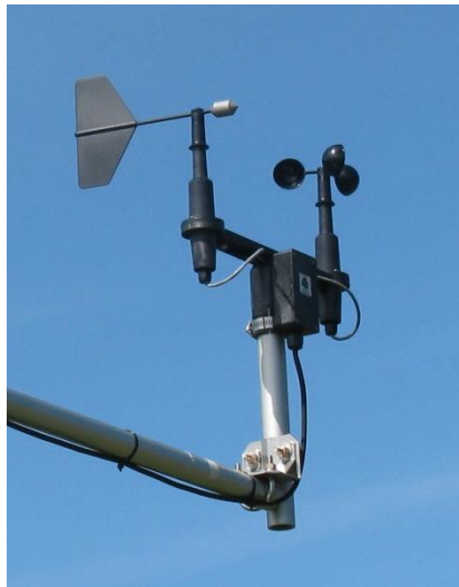
Figure 12: Wind Sentry Set as installed.
