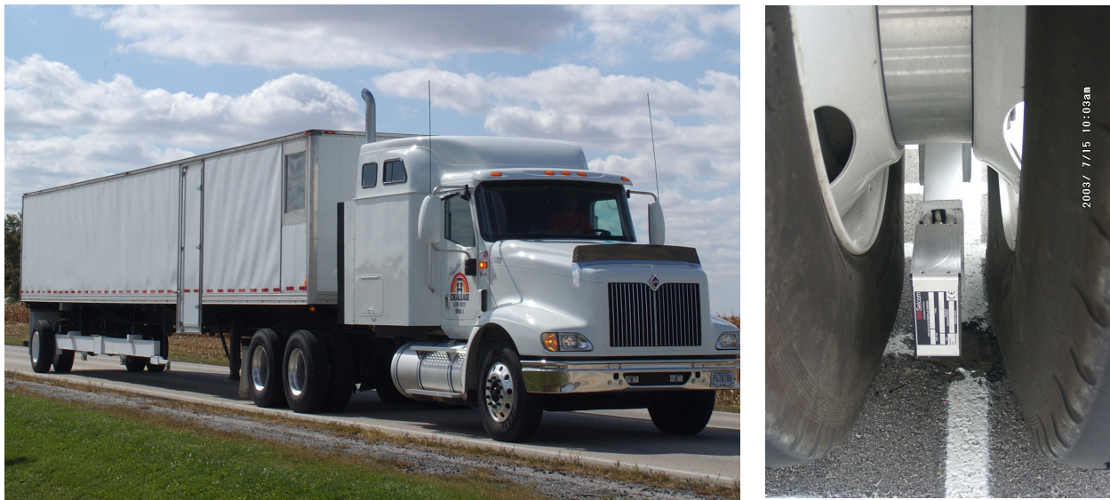
Figure 2. Overview of the RWD and a close-up of laser D between the dual tires.
