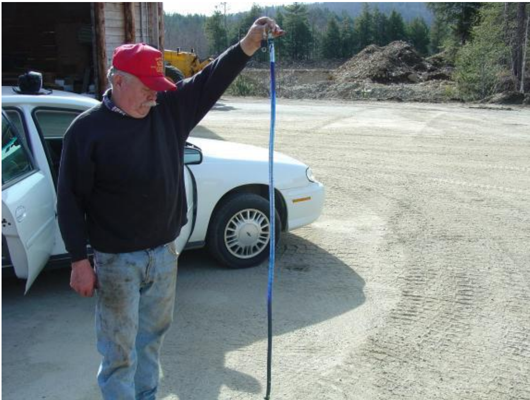
Figure 11: Frost tube with clearer colored frozen liquid in the top two-thirds and darker colored thawed liquid in the lower third.
