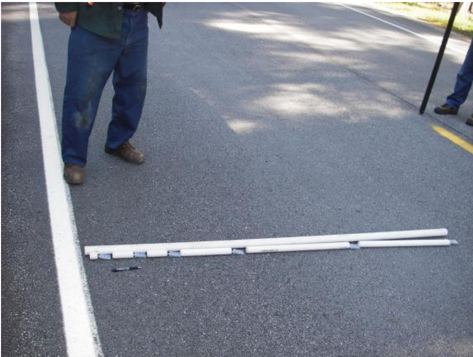
Figure 13: HOBO® setup (HOBO® and spacers in the foreground and the tube that holds the setup is in the background)
