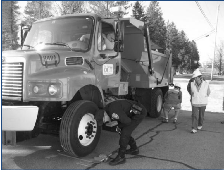
Figure 16: Trooper Huddleston (NH State Police) taking NHDOT wheel load measurements
