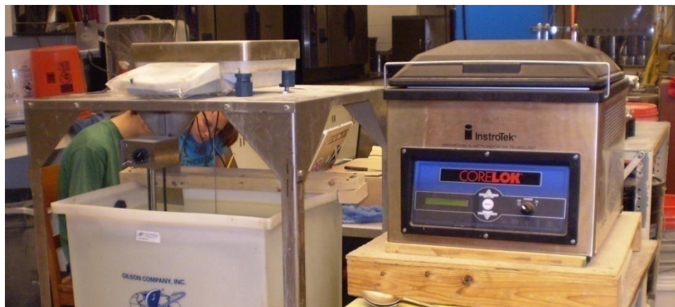
Figure 3-5: Corelok System Used to Determine Theoretical and Bulk Specific Gravities
