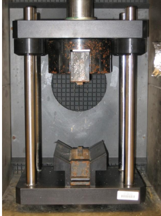
Figure 4-2: IDT Load Fixture inside the Temperature Chamber
