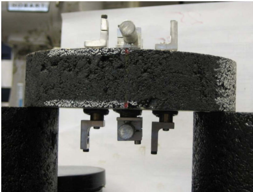
Figure 2.9: LVDT Brackets on Both Faces of the Sample
