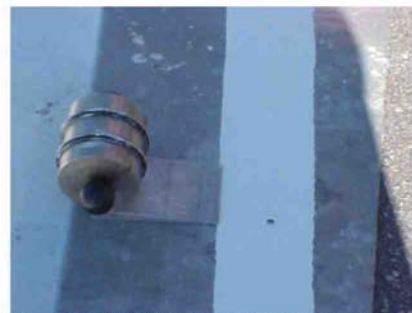
Figure13-d: ASTM D711 No-pick-Up wheel and ramn
