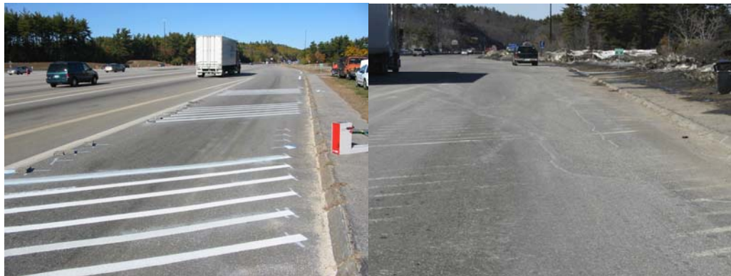
Figure 3: Traffic paint at the Hooksett test site. Left on October 29th 2002. Right on March 16th, 2003.
