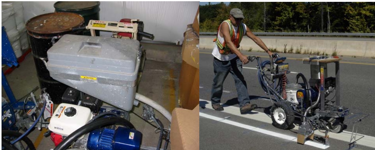
Figure 11: Unmodified sprayer with plastic bead hopper (left) and modified sprayer with SS bead hopper and wind deflectors in place.
