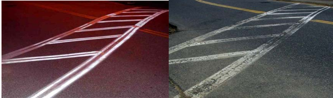
Figure 2: Traffic paint at the Durham test site. Left on August 2002. Right on May 8th, 2003.
