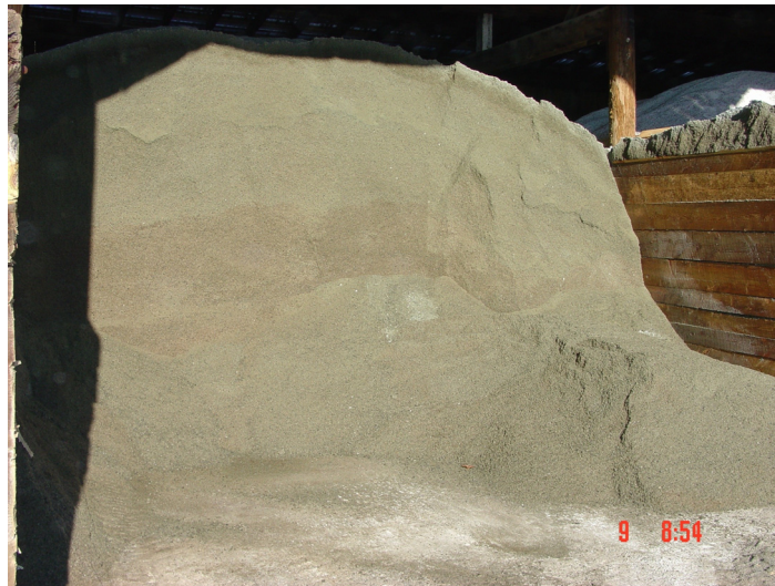
Figure 5: Leaching of Additive Observed in Bristol Stockpile
