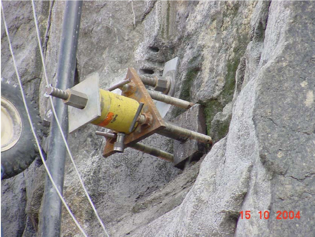
Figure 5. Lift-off Test for Prestressed Rock Bolts
