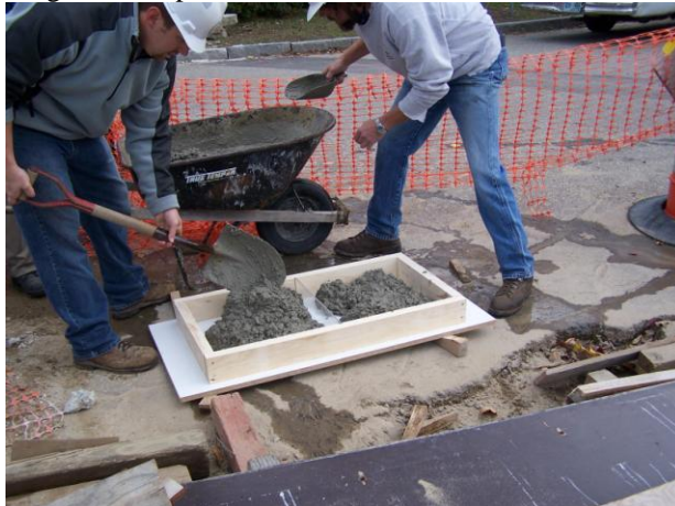
Figure 2: Preparation of test beam slabs on 10/17/2005
