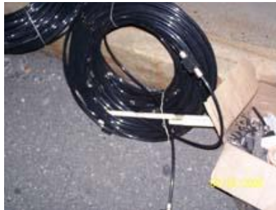
100 m rolls of supply tubing with micro nozzles mounted.
