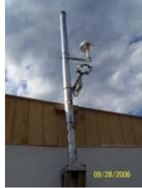
Roadway Weather Information System is installed at pump house. The system measures ambient air temperature, relative humidity and rainfall.
