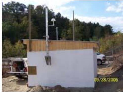
Roadway Weather Information System is installed at pump house. The system measures ambient air temperature, relative humidity and rainfall.
