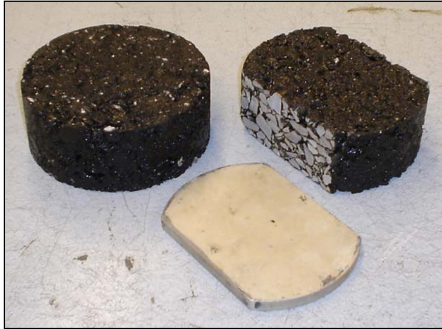
Figure 3.13: A Compacted Sample, a Brick, and the Cutting Template
