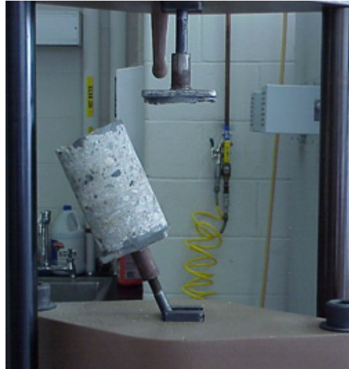
Figure C-2 – Core after failure in overpour
