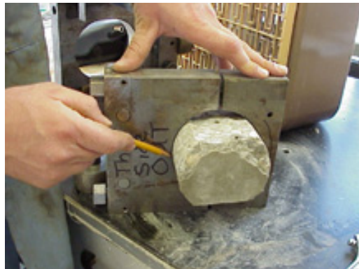
Figure A-5 - Core is marked for orientation
