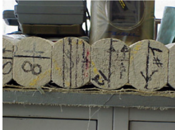
Figure A-2 - Trimmed deck cores ready for testing
