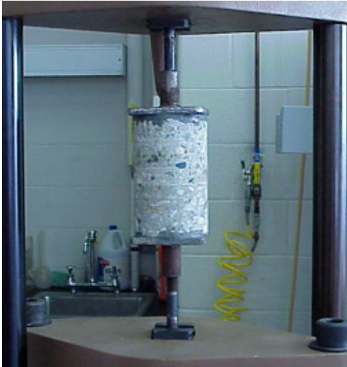
Figure C-1 – Core loaded for testing
