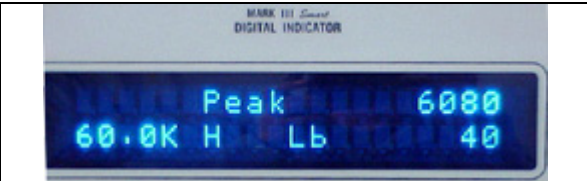
Figure A-9 - Typical display at failure
