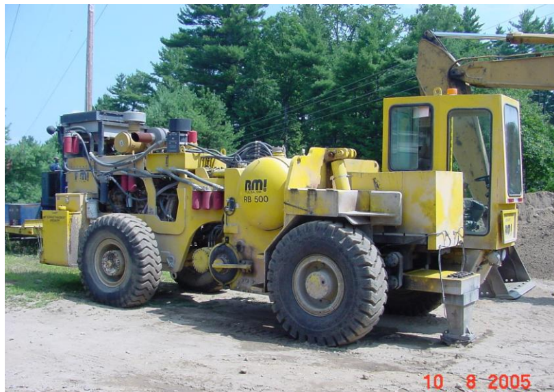
Figure 5 - Pavement breaker for rubblizing concrete
