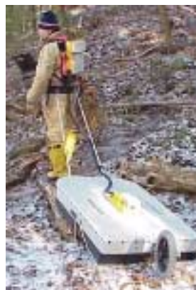
Figure 11: GPR unit fully assembled & being towed over the ground surface
