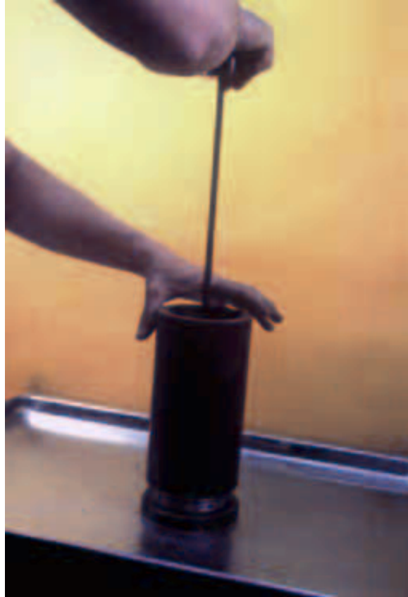
Figure A4. Extrusion of rings for 71-mm samples.
