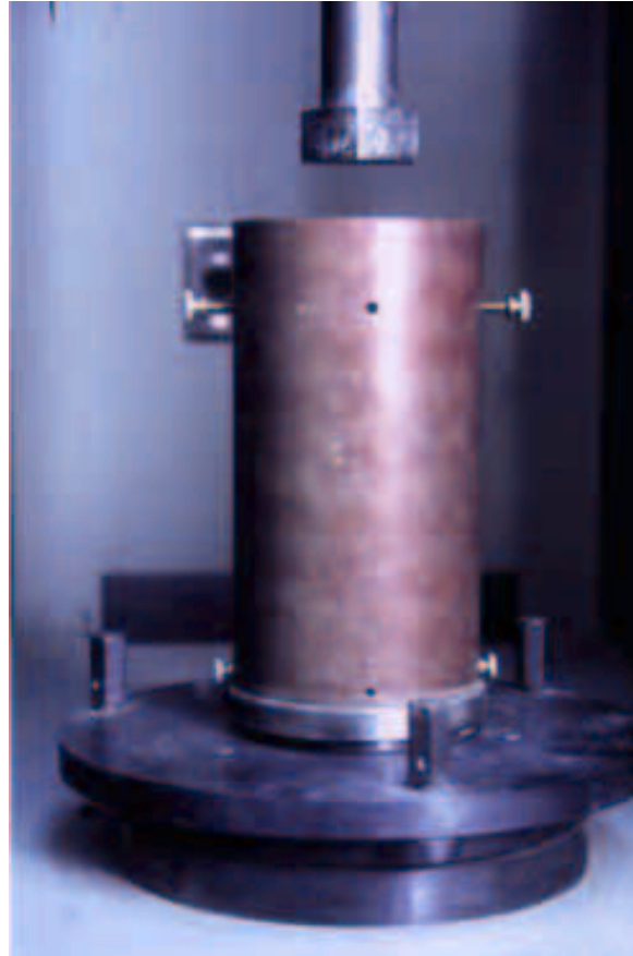
Figure A3. Apparatus in kneading compactor.
