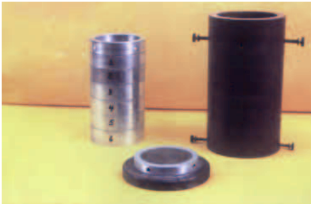
Figure A1. Split ring mold used for uniform density verification tests.
