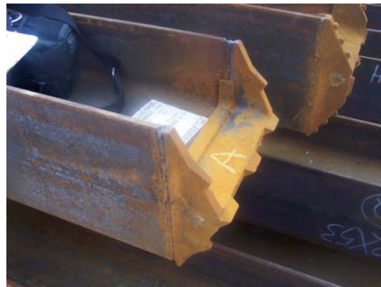
Pile Point A before driving
