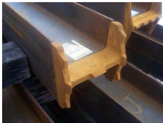
Pile Point I before driving
