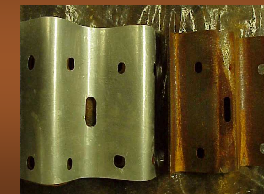
Zinc Insert — Pre Salt Fog Zinc insert on left
