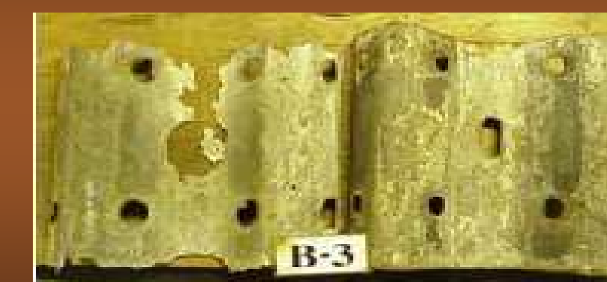
Zinc Insert — Post Salt Fog Sacrificed zinc insert on left—little damage to rail (Insides shown)
