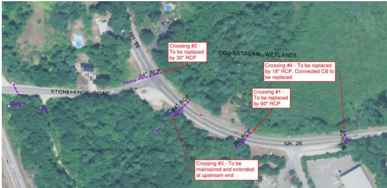
Figure 1: Pipe crossing locations
