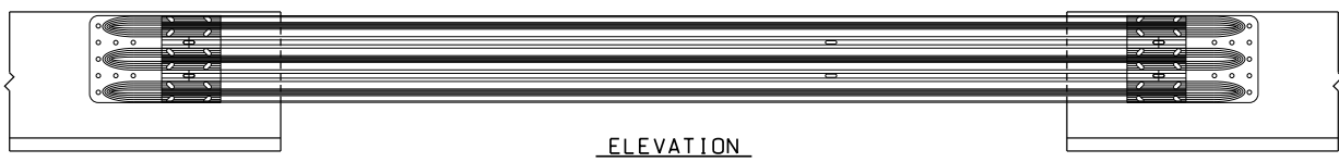
WORK ZONE BARRIER LAYOUT AT EXPANSION JOINT (PHASE 1 ONLY) N.T.S.
