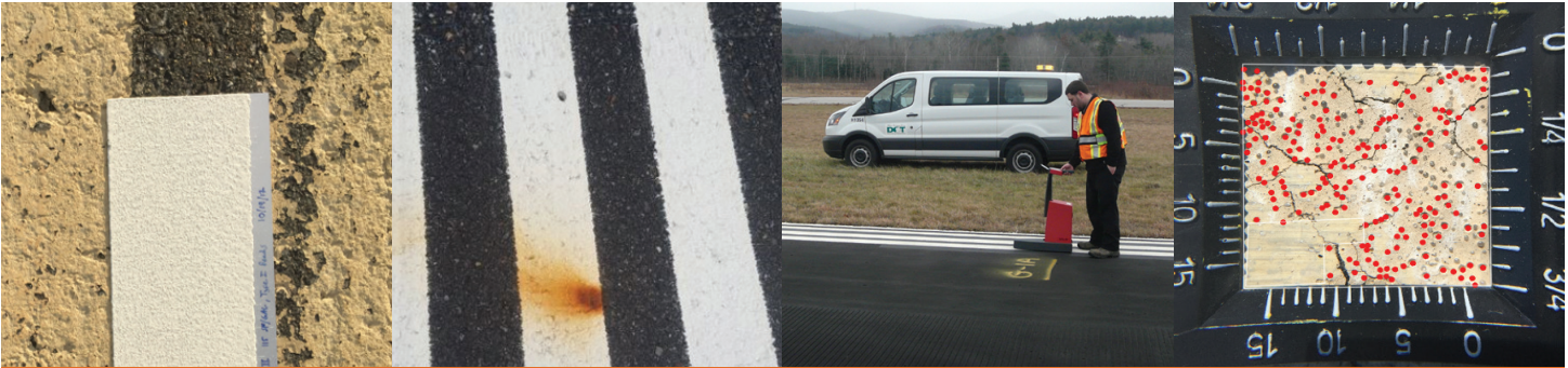
Magnified images of each study area were imported into CAD and the loss of beads were counted. Red dots are bead losses.
