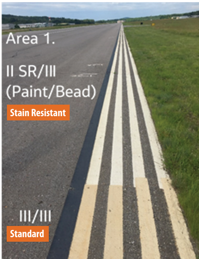
Paint color comparison made with original white control panels placed next to field stained paint.
