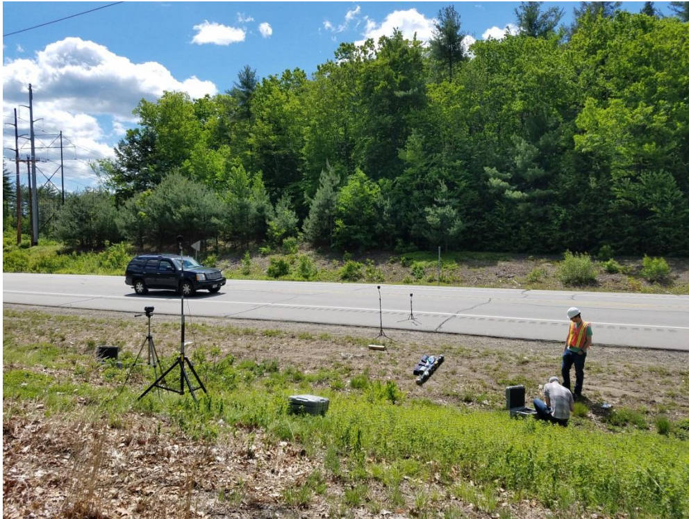
Site 1 – Microphone locations along southbound lane (near lane)
