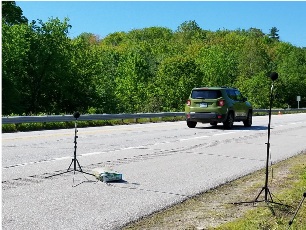
Site 5 – microphones at the 17-foot and 25-foot positions
