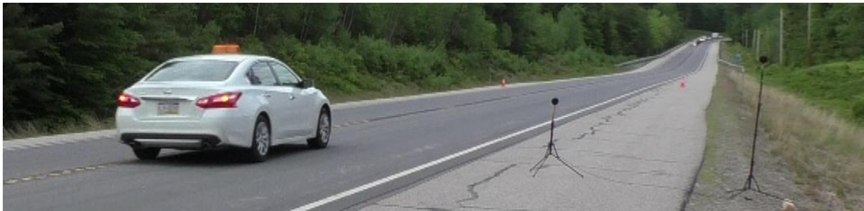
Figure 4 Continuous Vehicle Pass-by on the Center Rumble Strip (Near Lane) at Site 4 (Alton)
