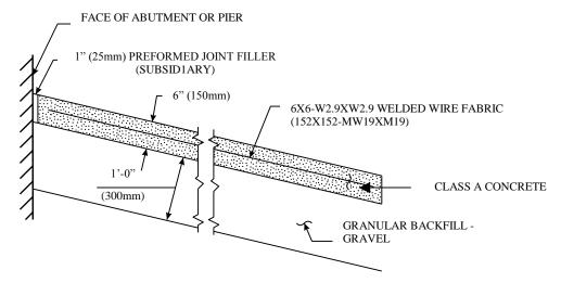
DETAIL FOR TYPICAL 4: 1 SLOPE OR LESS
