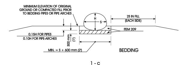
FIGURE 1 - STRUCTURAL PLATE PIPE AND PIPE-ARCH DETAILS
