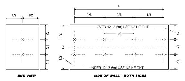
NOTE: WHEN "L" IS GREATER THAN 24 FEET (9 m), SPACING OF THERMOMETERS INDICATED BY (\*) TO BE APPROXIMATELY 8 FEET (3 M) ON CENTERS LONGITUDINALLY.
