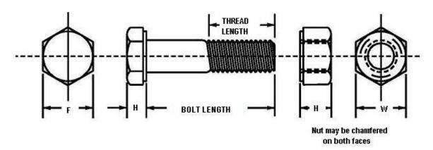
FIGURE 1 - HEAVY STRUCTURAL BOLT AND HEAVY NUT
