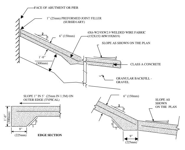
DETAIL FOR TYPICAL 6: 1 OR 4: 1 SLOPE TO A 2: 1 SLOPE
