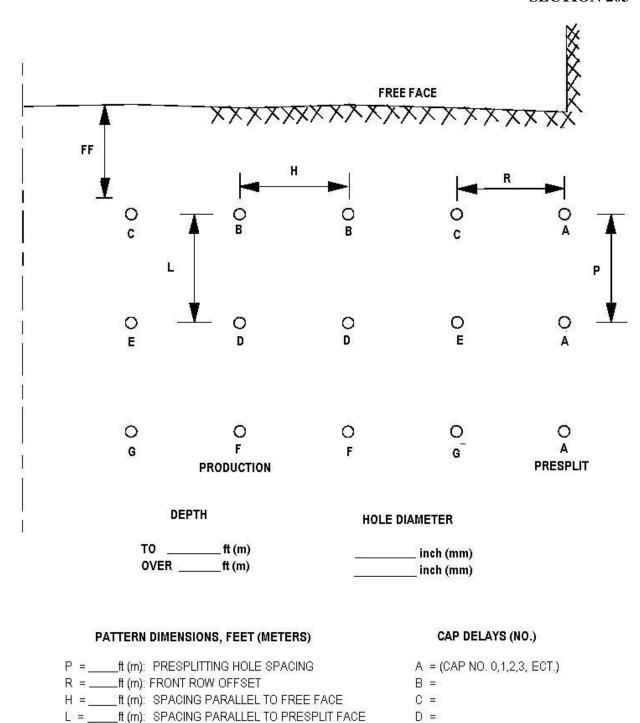
FIGURE 1 - TYPICAL BLASTING PATTERN
