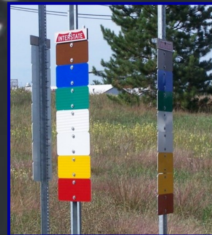
A Control Sign Pole was constructed at the Bureau of Traffic to monitor the loss of retroreflectivity of various sheeting types. Signs installed in the field concurrently with these control panels can be replaced when periodic retroreflectivity readings deem it necessary.
