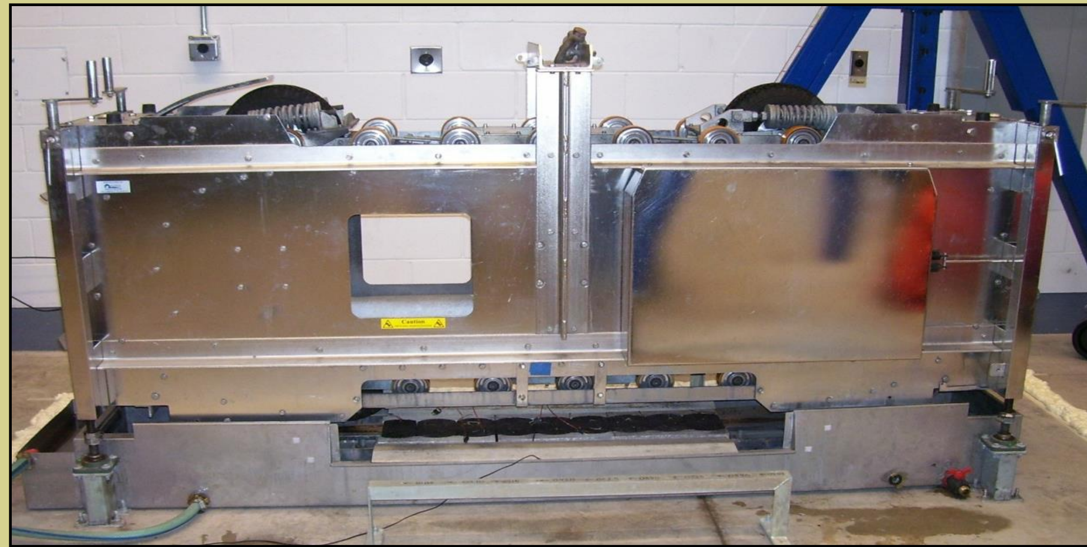
Figure 1: Third Scale Model Mobile Load Simulator
