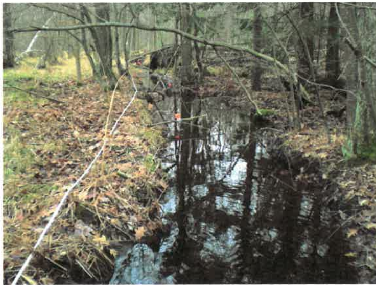
Figure 3-2. Upper reach of west side stream looking downstream from cross-section. Orange flagging notes bankfull stage and location of survey location for longitudinal profile. Photograph taken on December 2, 2009.
