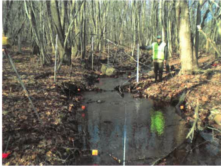
Figure 3-9. Lower reach of west side stream looking upstream from cross-section. Orange flagging notes bankfull stage and location of survey location for longitudinal profile. Length of stadia rod is 4.8 feet. Photograph taken on December 4, 2009.
