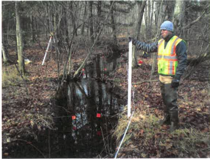
Figure 3-1. Upper reach of the west side stream looking upstream at cross-section. Orange flagging notes bankfull stage and location of survey location for longitudinal profile. Length of stadia rod is 4.8 feet. Photograph taken on December 2, 2009.
